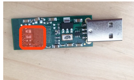
Fig.: Security-Relevant Signals in the top layer of the design / Security-Relevant Signals exposed using a scalpel. Note that several components were desoldered.
